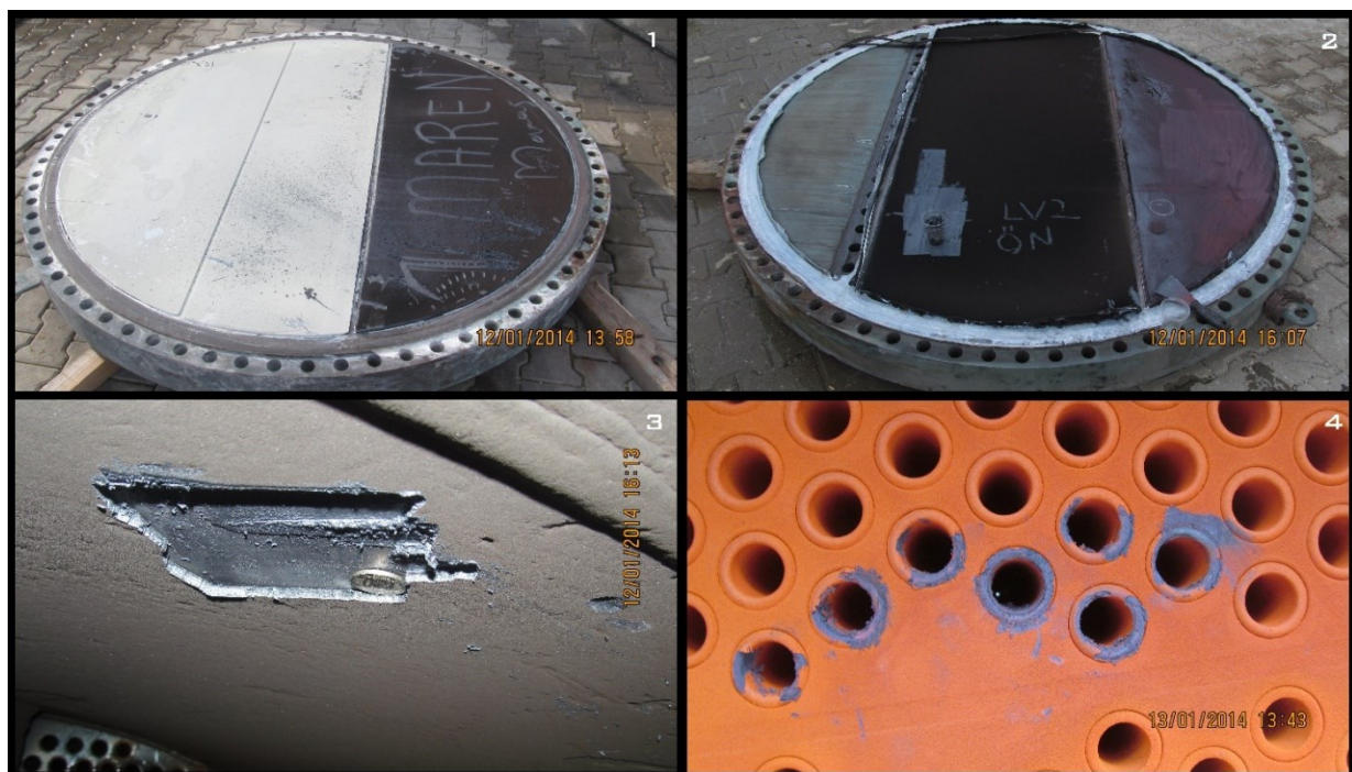
Figure 5: Scales encountered in Irem heat exchangers; 1: HP vaporizer, 2: LP vaporizer, 3: HP&LP vaporizer, 4: preheater last pass
