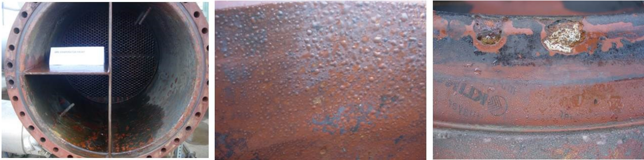
Figure 2: Surfaces of the ORC Evaporator front side after water jetting (left). Blister formation in heat exchanger cap (middle). Coating spalling and exposure of metal surface to the geothermal brine (right). After Scheiber et al. (2013a)
