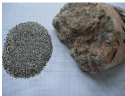
Figure 10: Host rock material of the Soultz granitic reservoir: Cuttings from GPK-2 (appr. 4775 m depth) and a piece of core from EPS-1 (1674 m depth), after Scheiber et al. (2013) and Scheiber et al. (2014).
