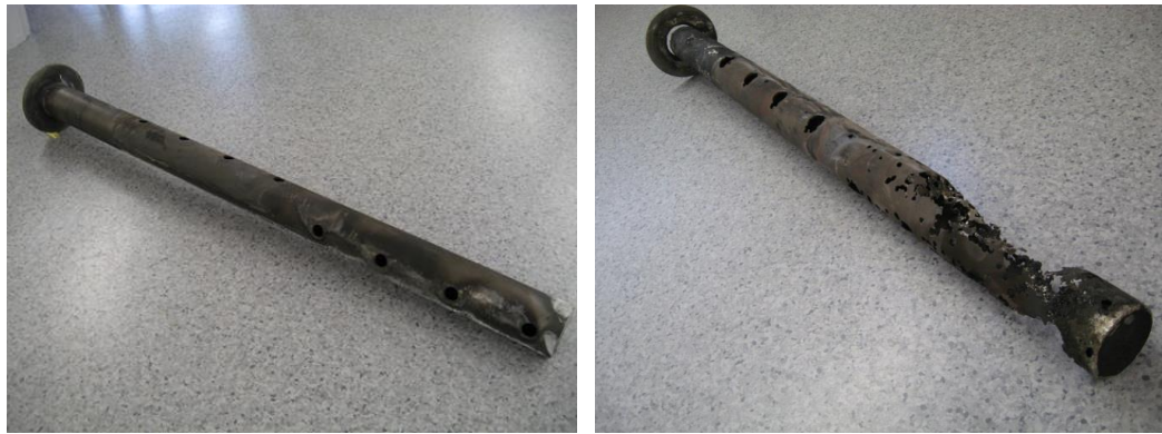
Figure 5: Before and after service photos of an H-276C injection quill at the Kawerau Geothermal Power Station where the quill is exposed to acid concentrations of 1-2% and temperatures of approximately 190°C, with some flashing occurring due to the exothermic mixing of acid with water.
