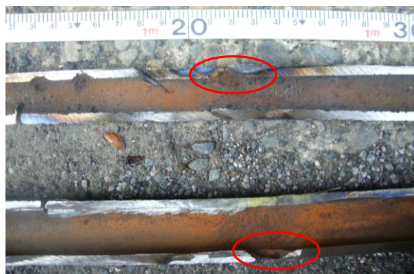
Figure 3: Pipe perforation at 2.2 m from the inlet header end plate (only 8.5 m of the 9.5 m long tube was recovered).
