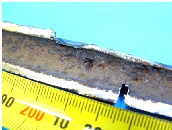
Figure 4: Small pits observed along the tube near the area of perforation of the removed tube section.
