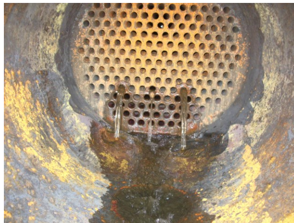
Figure 2: Heat exchanger exit header end plate view showing leaking tubes from perforations in a single row of tubes.
