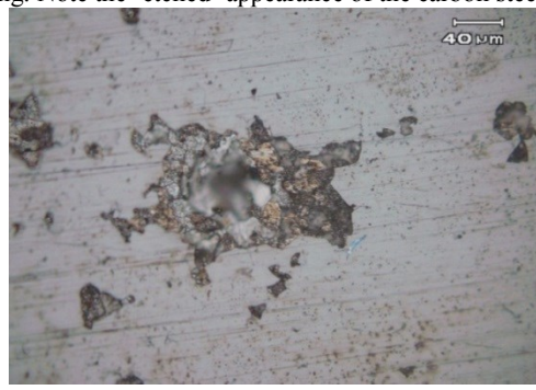
f) "Unscratched" arsenic coated coupon surface showing isolated deep pit within small area of damaged coating.
