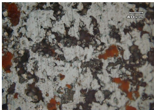
e) View of cleaned arsenic coated coupon away from the scratched area showing localised corrosion and retained areas of coating.
