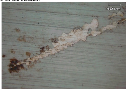
f) View of un-corroded carbon steel surface with pre-existing coating damage.
