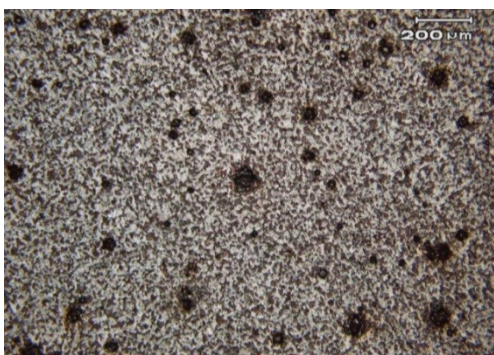
a) Optical image of general surface corrosion and localised pitting corrosion under brown precipitate.
