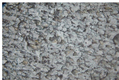
b) View of the cleaned carbon steel coupon showing roughened and 'etched' surface.
