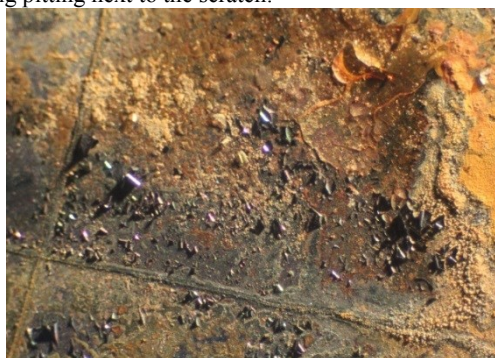
c) Close up view of as-exposed surface of "scratched" arsenic coated coupon showing coating spalling.
