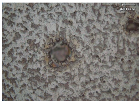
b) Close up view of pitting corrosion and 'etched' general corrosion appearance of carbon steel surface.
