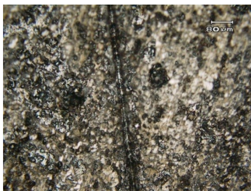
a) View of cleaned 'scratched' antimony coated coupon surface showing pitting next to the scratch.
