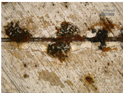
a) View of cleaned 'scratched' antimony coated coupon surface showing pitting corrosion next to and on the scratched area, surrounded by retained coating.
