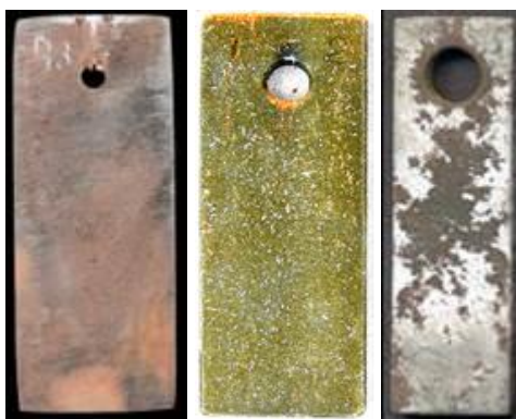
Figure 2: Carbon steel after 6 months exposure in artificial waters; left: MB, 150 °C; Center: LHD, 175 °C; right: NGB, 150 °C.
