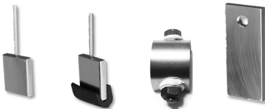
Figure 1: Specimen design for electrochemical, crevice corrosion, SCC and exposure tests.
