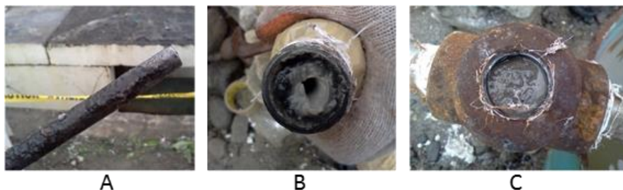
Figure 7: KN2D pH modification side-stream test pipe inspection. Inspection of the pipe segments after the dosing activity showed heavy silica deposition from the dosing point towards the pipe outlet. Heavy silica deposits were noted upon inspection of the injection probe (a), pipe segment after dosing point (b), and pressure gauge tee (c).
