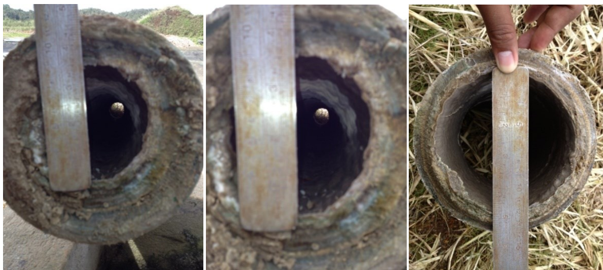
Figure 3: Depositions at the first TW line inspection lines
