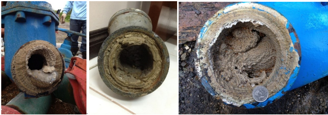
Figure 4: Massive depositions at joints, elbows, and valves
