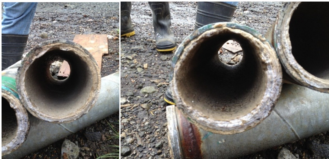
Figure 5: Redundant line used for the dosed brine fluid
