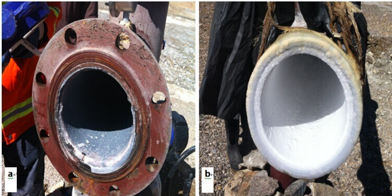
Figure 2: Effects comparison chart of spray tests in ZK11 geothermal well. (a) Under the condition of pressurizing 0.5 relative to the atmosphere, the scale thickness is less than 1 mm after five days. (b) At the same time, under the condition of non-pressurization, the scale thickness is 10 mm.
