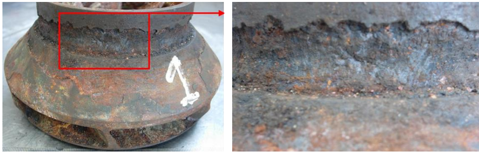
Figure 3: Views of wear caused by "sand-cutting" of impeller No.1 of the pump removed in May 2012
