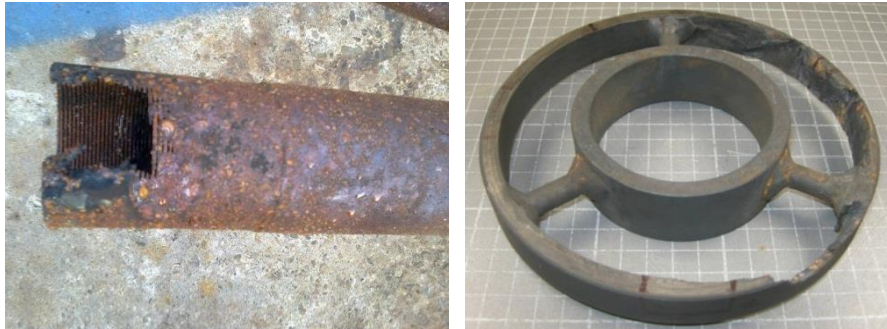
Figure 4: View of the leaking driveshaft-enclosing tube and of one centraliser damaged by stress corrosion and removed in November 2011
