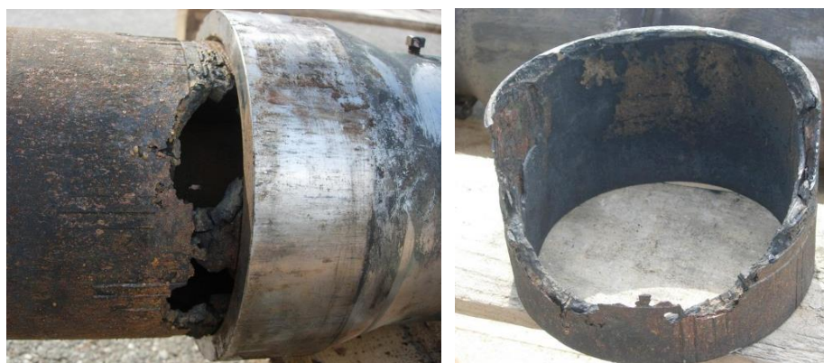
Figure 10: View of the production tube connected to the pump assembly before dismantling (left) and after (right)
