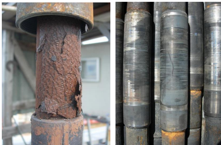
Figure 9: View of oxide and carbonate layer on the shaft (left) and of wear observed on several drive shaft bearing sleeves (right)
