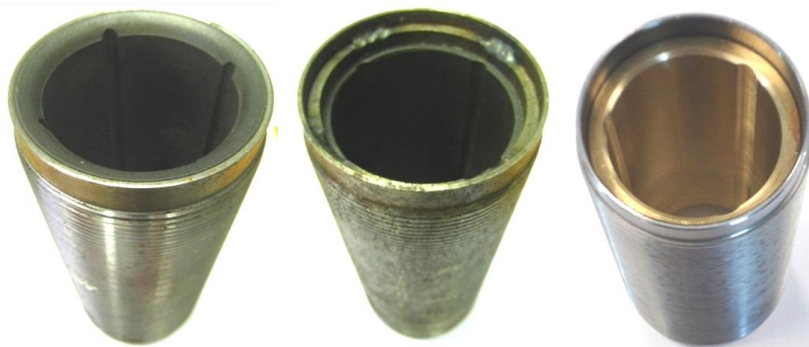
Figure 5: View of the different lineshaft bearings tested in Soultz: standard Icelandic (on the left), with welded rings and carbon-graphite Teflon insert (middle) and bronze bearing insert (on the right)
