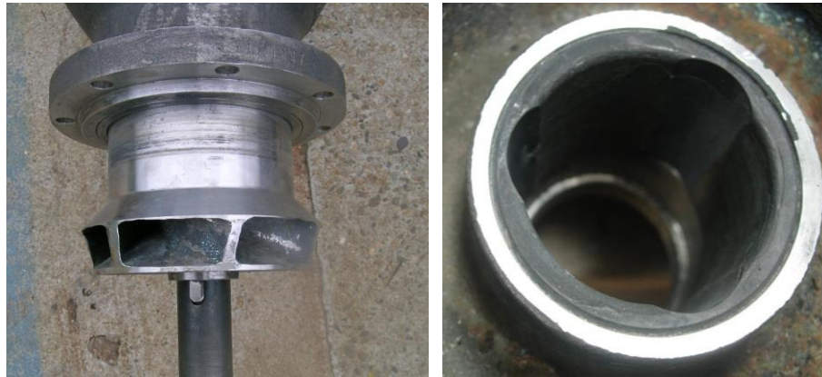
Figure 11: View of the top impeller after cleaning (left) and of the top stator bowl bearing (right)
