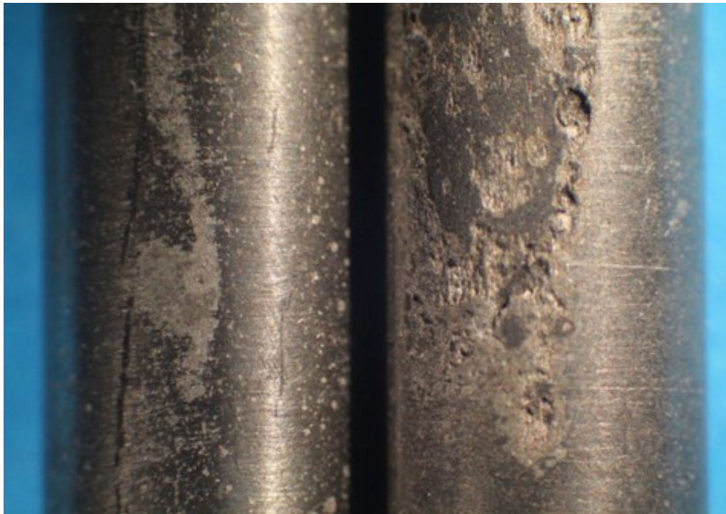
Figure 1: Illustration of localised corrosion under reductively deposited heavy metal scale at pH 6 (left) and pH 5(right) as described by Lichti and Brown, 2014.
