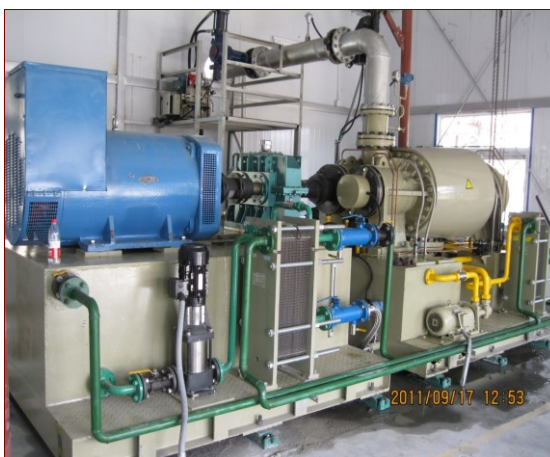
Figure 3: The testing screw expander generating unit in YangYi
