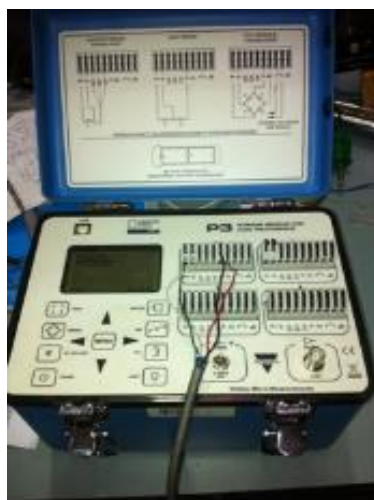
Figure 9- Vishay strain indicator used for taking the impulse force
