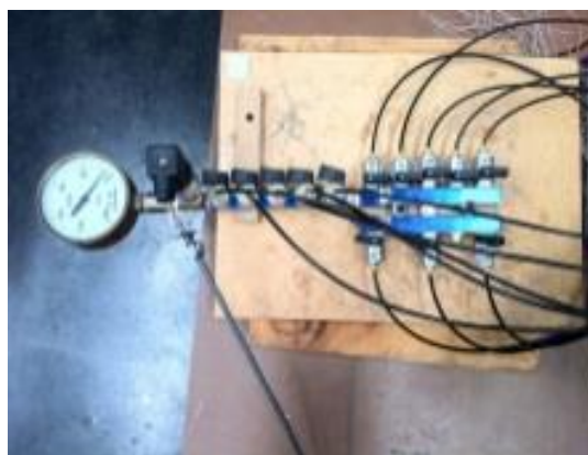
Figure 10- Manifold used for measuring the pressure at each location along the nozzle
