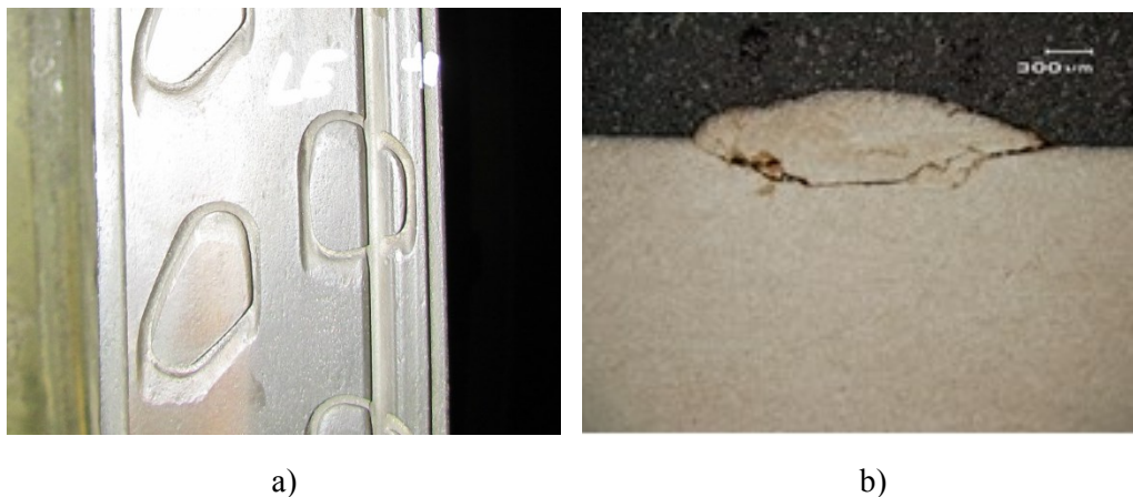
Figure 4: a) Groove cut into coverband by diaphragm seal and b) area of material stiction and subsurface cracking
