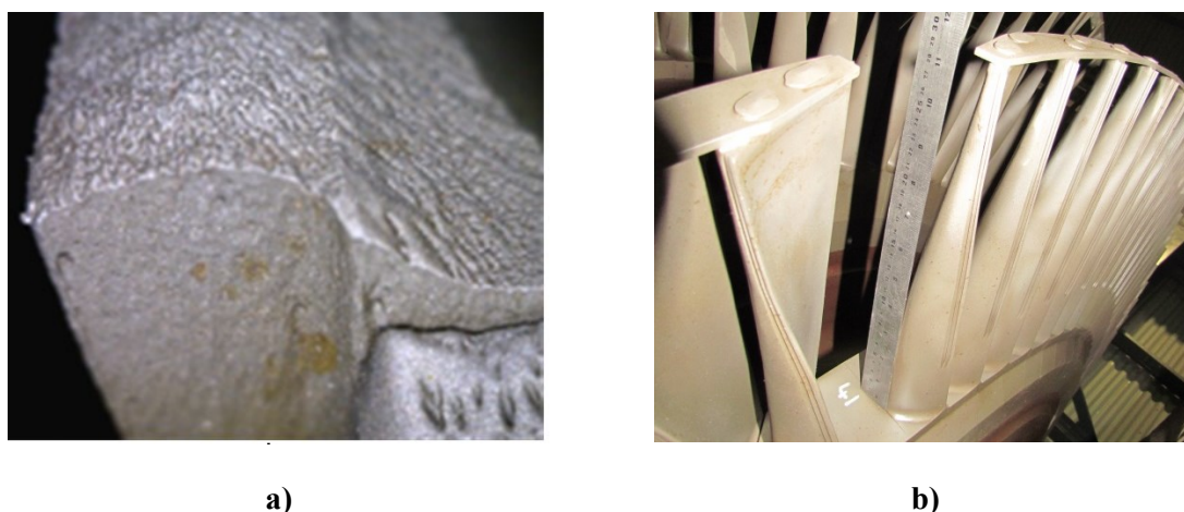
Figure 7: a) Water impact erosion on leading edge of rotating blade and b) water drainage grooves on suction side of leading edge.
