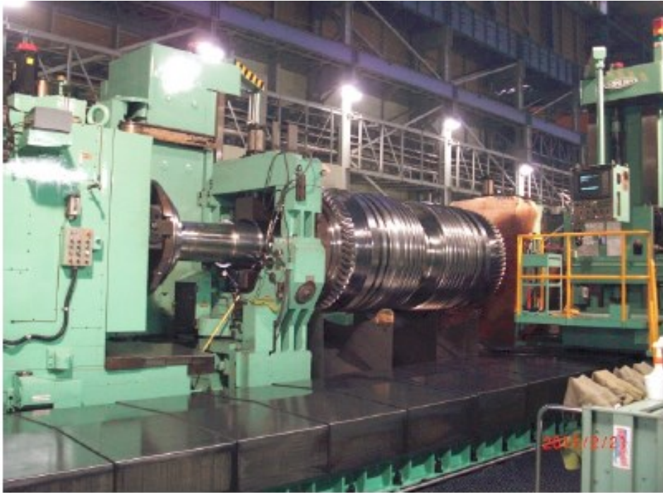
Figure 8: Machining process of turbine rotor in Fuji Electric factory.
