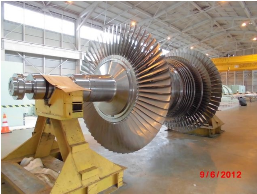
Figure 10: New turbine rotor in Wayang Windu Geothermal Power Plant.
