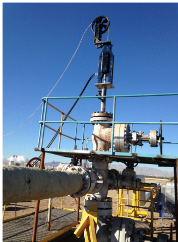
Figure 7: Acidification in silica scaled well in Cerro Prieto.
