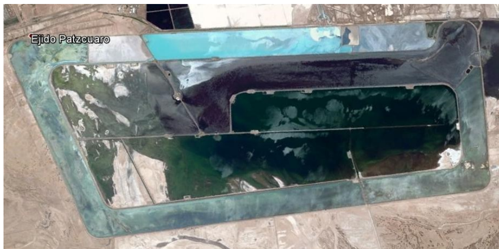
Figure 8: Evaporation Pond of 18km 2 with a maze arrangement.
