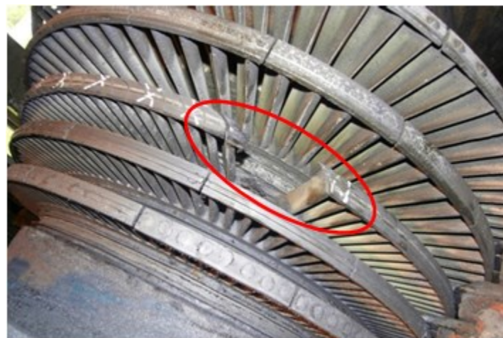
Figure 8: Some rotor blades were damaged
