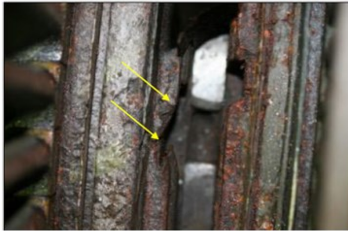
Figure 7: The turbine rotor drum was damaged.
