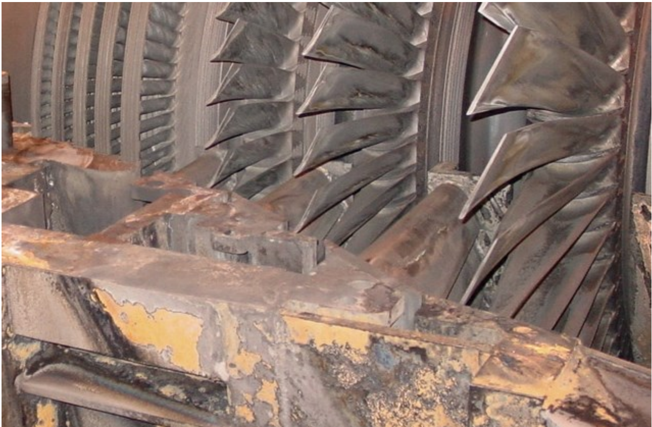
Figure 1: Turbine with top casing removed. Steam inlet is on left with condenser on the right. This is just half of a double ended rotor. The fixed blading vanes direct the steam in the opposite direction to the rotor blades. The slot for the interstage drain can also be seen just behind the second to last set of rotor blades. The components oxidize rapidly on exposure to air.
