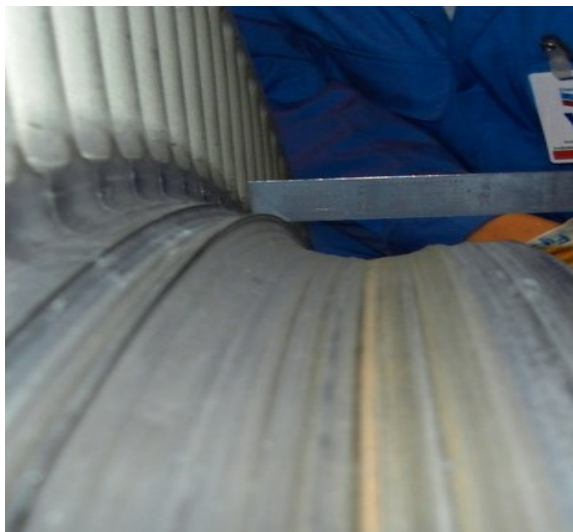
Figure 11: Rotor abrasion caused by deposition from mineralized water flow through the first stage nozzles.
