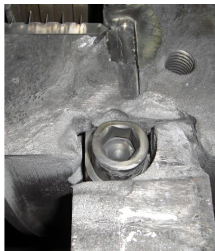
Figure 8: Steam damage across halfjoint sealing faces of the stationary blading sets. Steam flow right to left.
