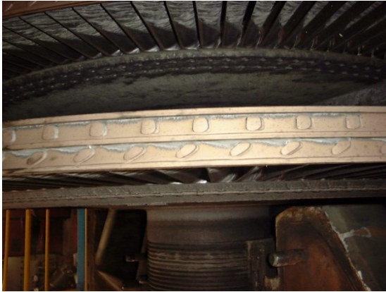
Figure 13: Blade tenon leading edge erosion from silt laden condensate. The rotor turns left to right. Wash lines of deposition can be seen on the upstream blading.
