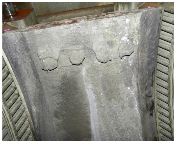
Figure 12: Rotor damage in figure GG caused by deposition on the annular cavity like that shown here. The steam is generally so wet that there is little if any deposition in the nozzles. The rotor damage root cause is poor separation coupled with excessive wash water flow and ineffective demisters.
