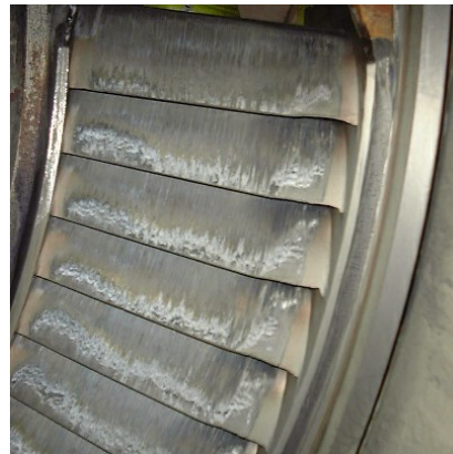
Figure 16: Erosion of trailing edge of diaphragm vanes caused by debris in steam. The rear edge should be straight
