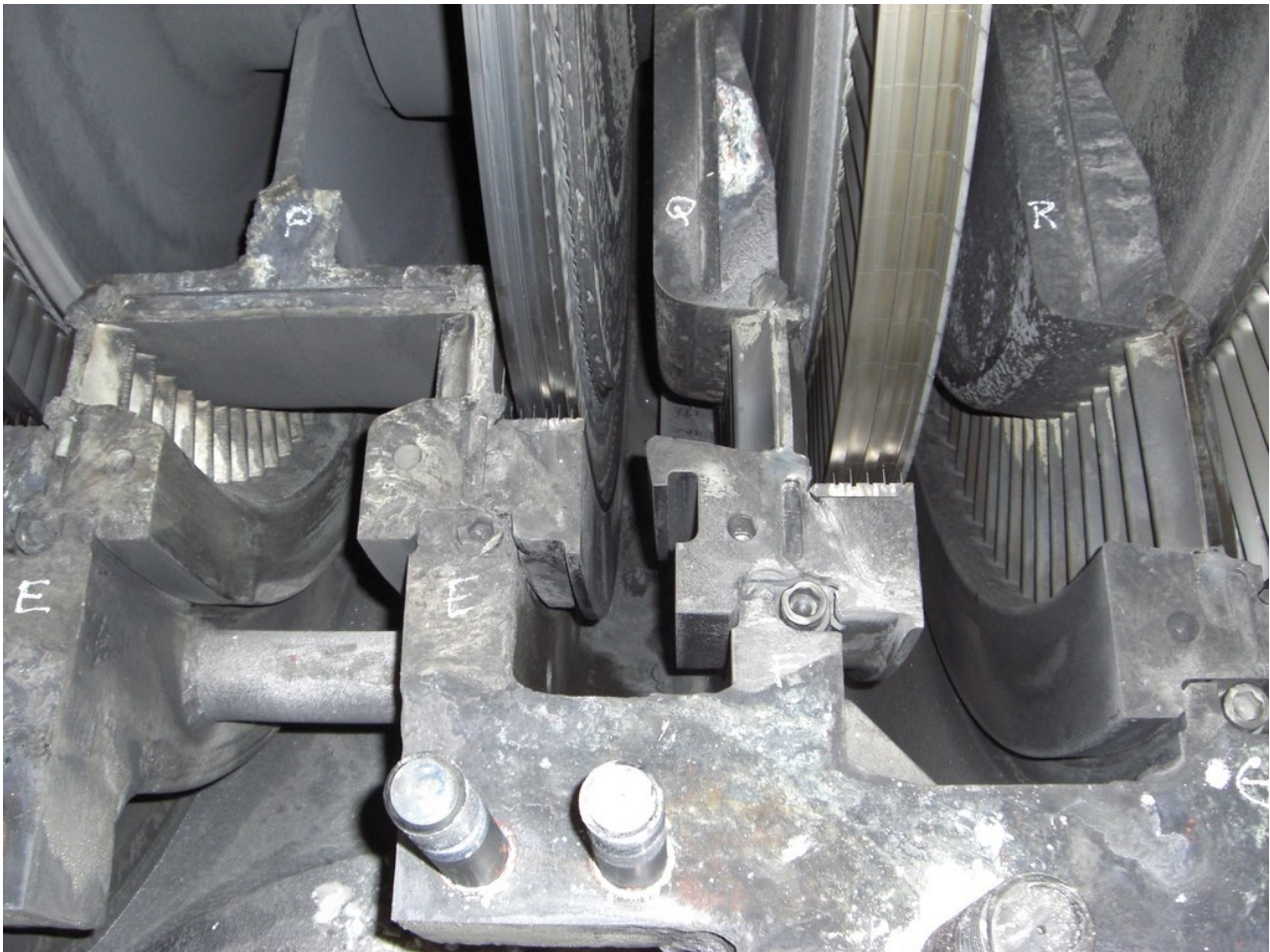
Figure 2: Turbine detail. The steam enters the cavity on the left and passes through the sets of stationary and rotating blades. The thin sealing strips on the trailing rings of the diaphragm stationary blades are to minimise the steam bypassing the rotor blades. The cavities between the diaphragms have drainage to allow water to be removed.
