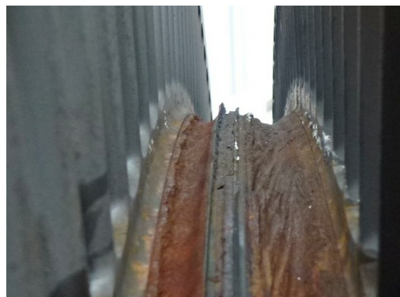
Figure 6: Rotor erosion from water trapped in the interstage area. There were originally thin stainless iron sealing strips in this region to prevent steam bypassing the fixed blading, of which only the remnants of two remain.
