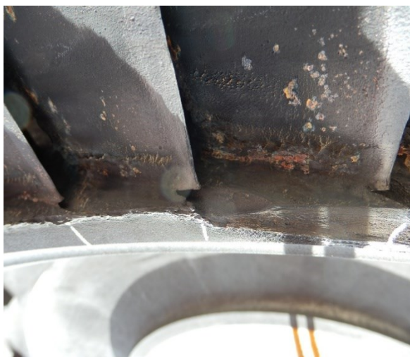
Figure 7 Water erosion damage on exhaust side of first stage nozzle inner port wall. This region is supposed to be superheated steam.
