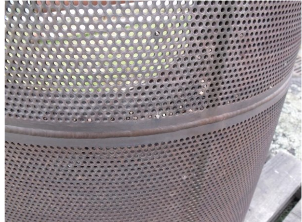
Figure 14: Rocks jammed in a steam strainer. This was downstream of a demister.
