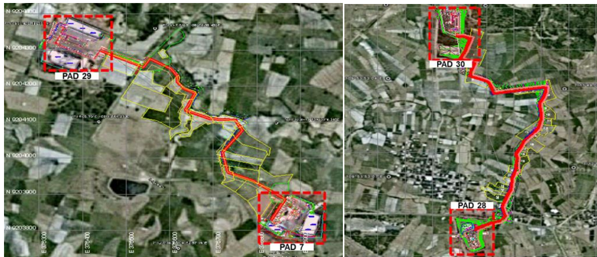
Figure 5. Pipeline route along 3 km connected tie-in wells to existing gathering system.
