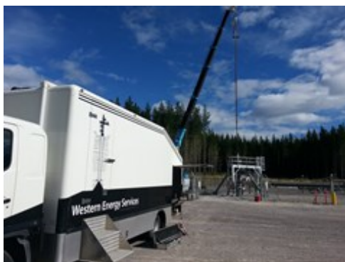
Figure 1: Wire line unit with 0.108" slickline, 25 tonne crane and approximately 21 m of lubricator during a survey of a 750 t/hr well
