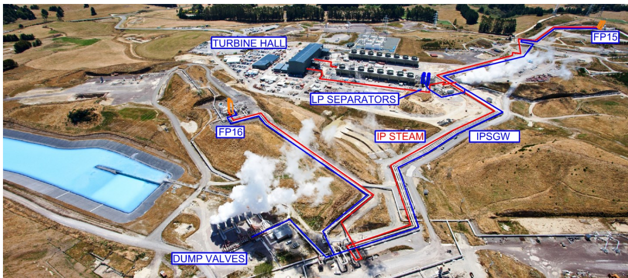
Figure 1 Te Mihi development viewed from the south during construction. Te Mihi station center, FP15 top right and FP16 center left. Separated Water dump valves bottom. IPSGW IP steam lines as shown.
