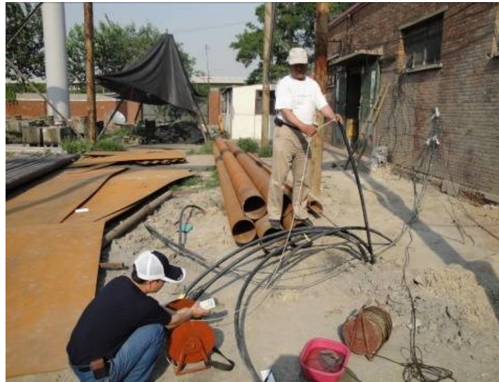
Figure 13: The measuring line in and outside of the PE pipe
