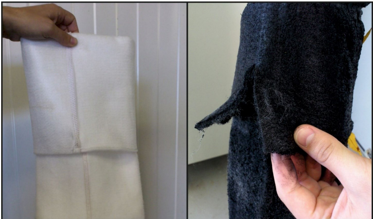
Figure 4: Filter before (on the left) and after (on the right) usage – with biofilm
