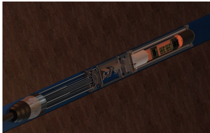
Figure 8: Picture of an early model of the COBOLD-probe, sliced for an inboard-view.
