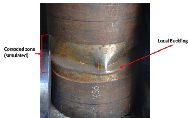
Fig. 8. Local buckling produced by external corrosion on casing: experimental results
