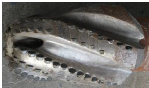
Figure 2: Exemplary used PDC formation window mills
