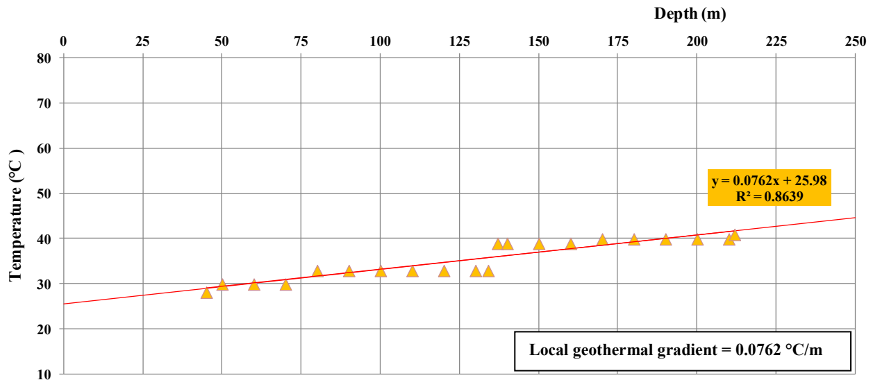
Figure 10: Evolution of the temperature in depth in the granitic massif in the area of Longroiva based on records of the AC1A borehole, as it was being drilled in 1999.
