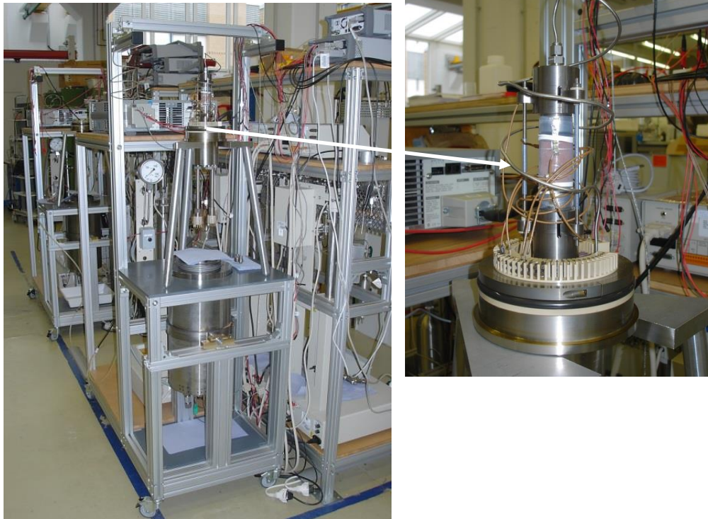
Figure 7: Rock physical flow-through apparatuses at GFZ-Potsdam to be transformed into devices for thermophysical measurements on fluid properties (viscosity, electrical conductivity, and sonic velocity).
