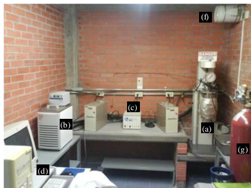
Figure 2: Experimental system used in the WRI experiments: (a) Parr® reactor; (b) Cooling bath and pumping module; (c) Analytical interface controller; (d) Data acquisition system; (e) Helium gas reservoir; and (f) Hot air extractor.
