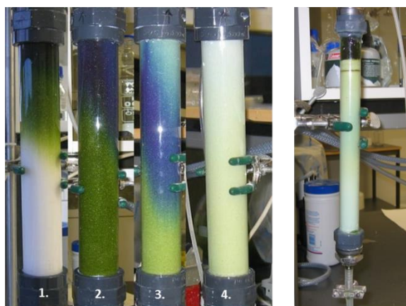
Figure 7. Left: Separation of C-PC in a column at different stages in chronological order: (1) at early stage of the loading, (2) after loading with 190 ml crude extract, (3) after flushing with 2.2 l of brine solution (25% BL-salt in deionized water), and (4) after elution with 2.0 l deionized water. Right: column with sintered BL-silica after loading and subsequent flushing with brine solution. Apparently no C-PC was retained.
