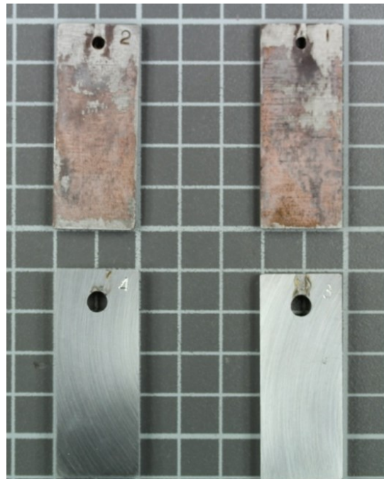
Figure 2: Reaction of carbon steel (top) and duplex steel (bottom) with saline copper(II) chloride solution. Native copper precipitation is clearly visible on the carbon steel samples.
