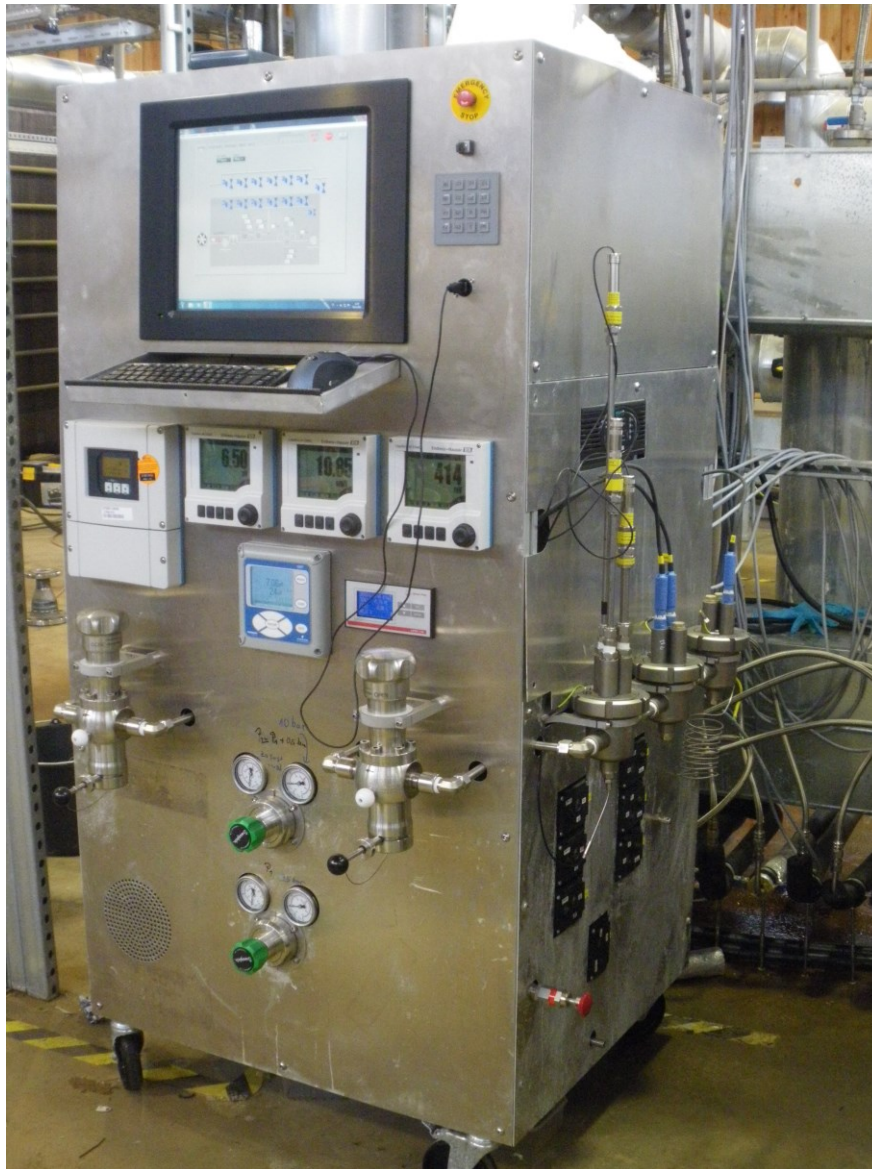
Figure 3: FluMo-1 as installed and operational at the geothermal research platform Groß Schönebeck, Germany. Control and data acquisition system (top). Sensors, analyzers, and fluid samplers (centre). Fluid pump and cooling circuit (bottom).
