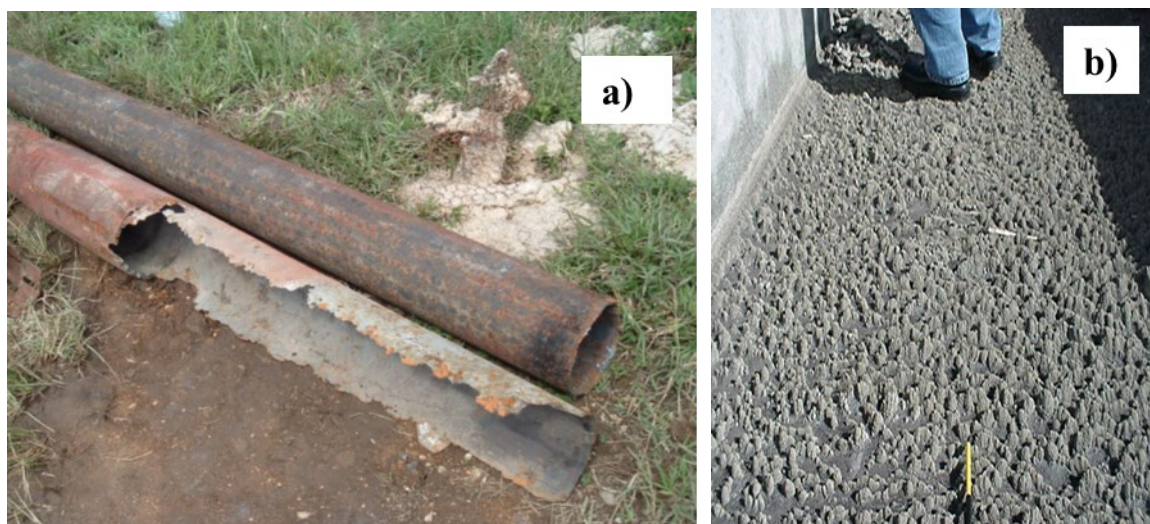
Figure 5: Problems related to acidic fluids, a) casing in acidic conditions, PGM-02 b) Deposits of silica in the PGM-07 channel.
