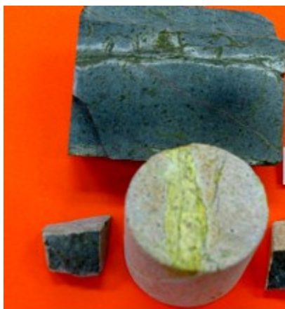
Figure 4: A fragment of core C, before acid treatment, with a vein sealed by quartz and epidote. After reaction in acid solutions the cylinder shows a bleached surface and no dissolution of quartz and epidote. The size of the cylinder is 3.5 cm of diameter and 4 cm height.
