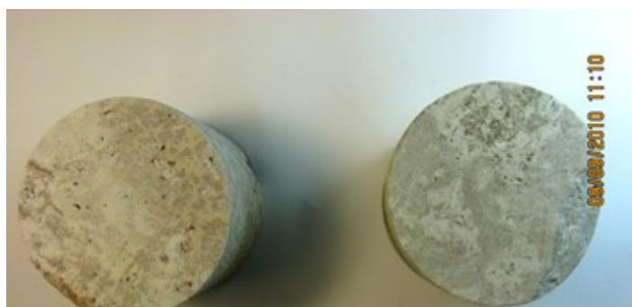
Figure 5: At the left a fragment of core B after acid treatments in the laboratory; at the right a fragment of core D as it is, without any acid treatment in the laboratory.
