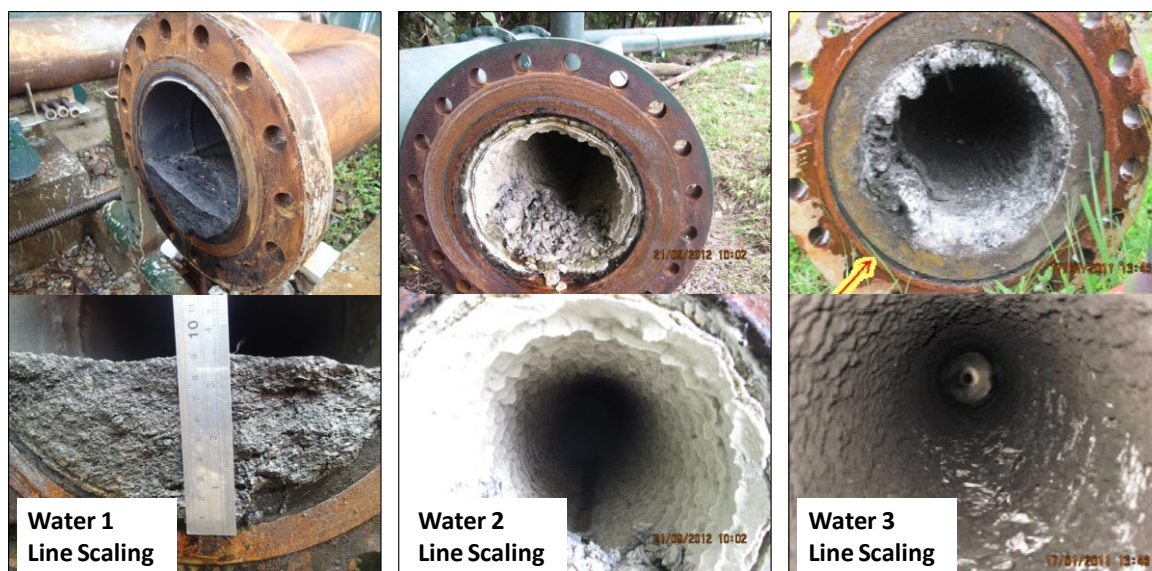
Figure 1: Fe-oxide/sulfide (left) and am. silica (center and right) scales documented in the geothermal water pipelines.
