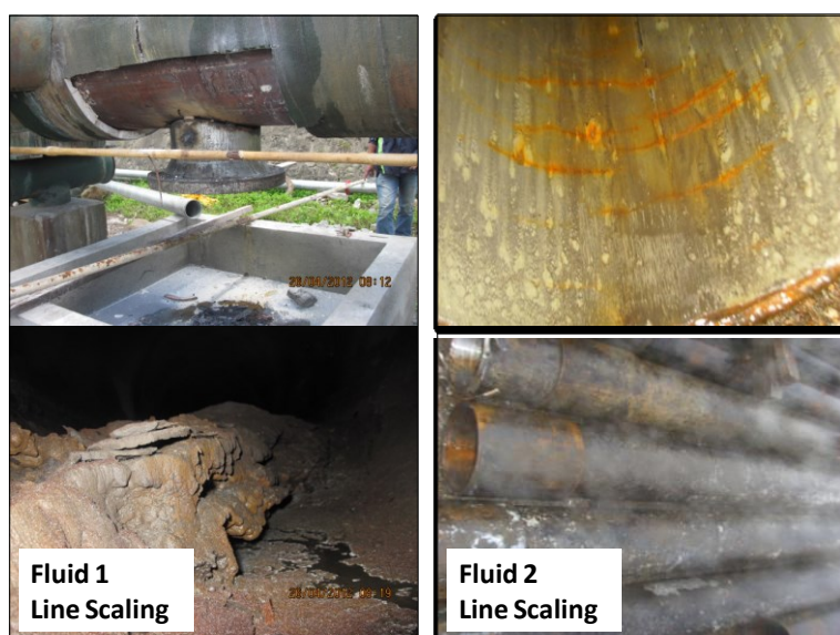
Figure 2: Fe-oxide/sulfide scales documented in Fluid 1 (left) and Fluid 2 (right) in the geothermal two-phase pipelines.
