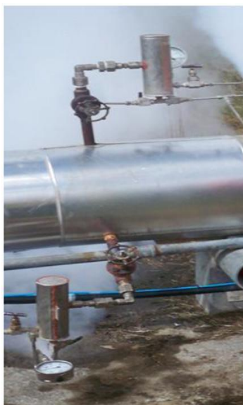
Figure 6. Picture showing the required instrument used for sampling a two-phase production well.
