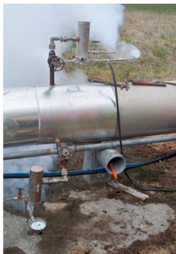
Figure 9. Single cyclone Weber separators are installed at the top for gas sampling and at the bottom (45° angle) for water sampling.
