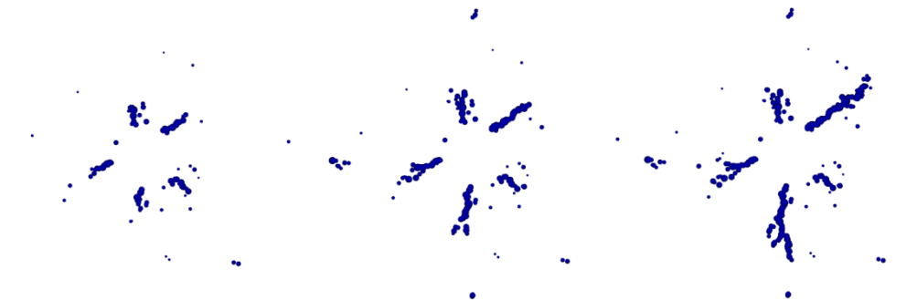
Figure 4 Accumulated fracturing event distribution. Tensile fractures are dominant in the process of the crack initiation and extension.
