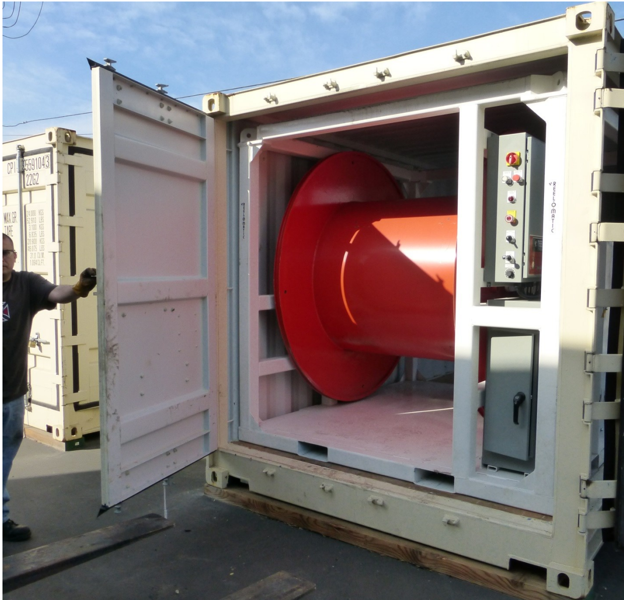
Figure 10. The electro-hydraulic spool especially developed for the tube containing the fiber optic fibers.
