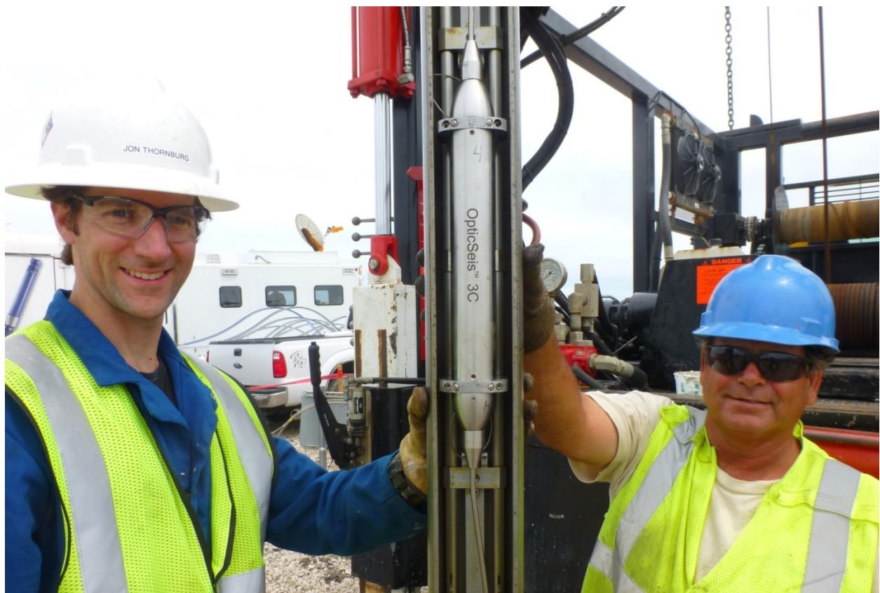
Figure 15. The deployment system and the pod with fiber optic sensor used for a field survey.
