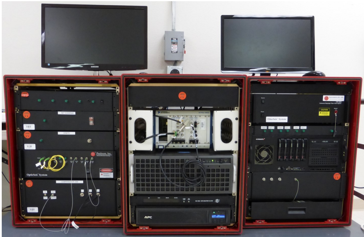
Figure 9. Optical Interrogator for Paulsson OpticSeis™ system.
