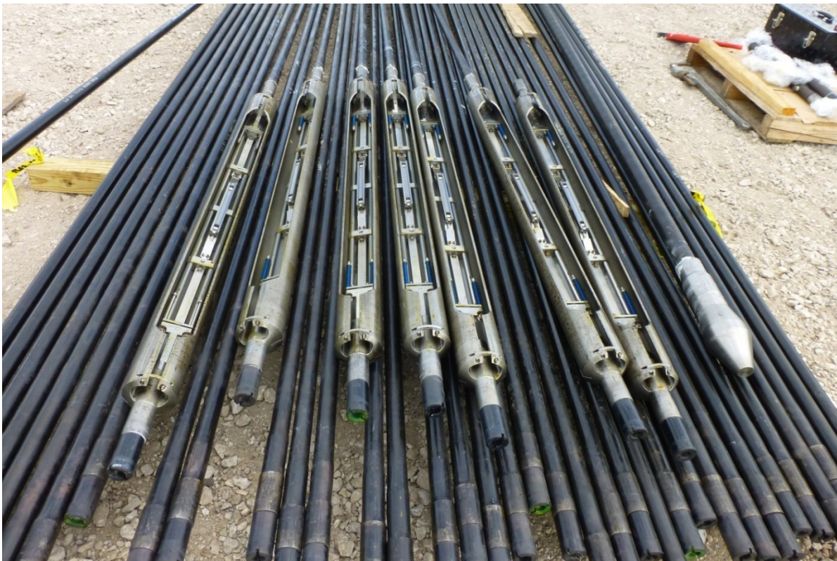
Figure 14. The drill pipe and the sensor pod housings used for the fiber optic seismic sensor system test survey.
