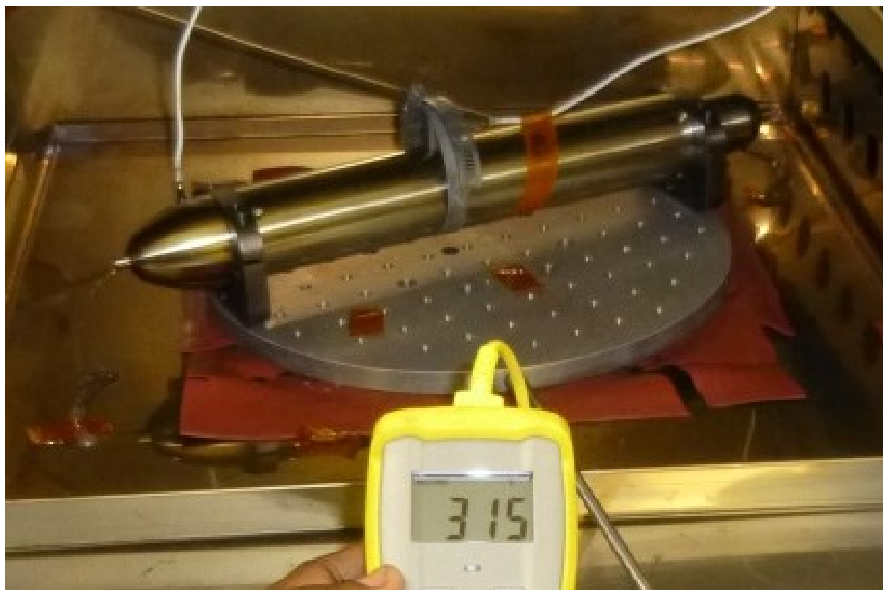
Figure 5. This photo shows the 3C sensor pod inside a high-temperature oven at a measured temperature of 315°C.
