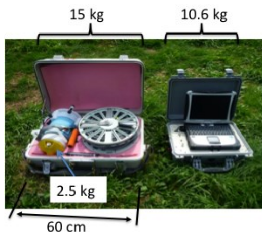
Figure 4: SQUITEM-3 magnetometer (left) and receiver system (right) (Sugisaki et al., 2013)
