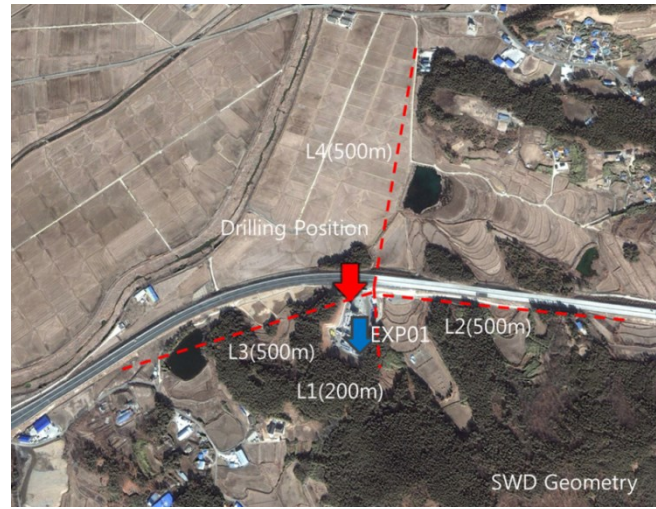
Figure 1: Geometry of the SWD survey in the vicinity of the geothermal well in Pohang, Korea, 4 radial seismic survey lines were deployed around the geothermal well (survey line 1 is extended 200 m and the other survey lines extended to 500 m using a 14-Hz geophone with 10 m interval and three-axial geophones were also deployed in every 50 m, a three-component borehole accelerometer is installed at EXP01 which is 150 m deep near the geothermal well for micro-seismicity monitoring.)
