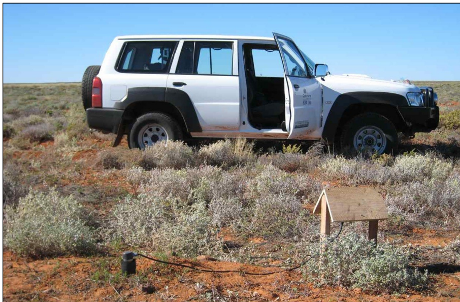
Figure 9: A Heat Needle (foreground) deployed in South Australia. The one meter long power and communications cable runs from the underground sensor string to the control box housed within beneath the sunshade.
