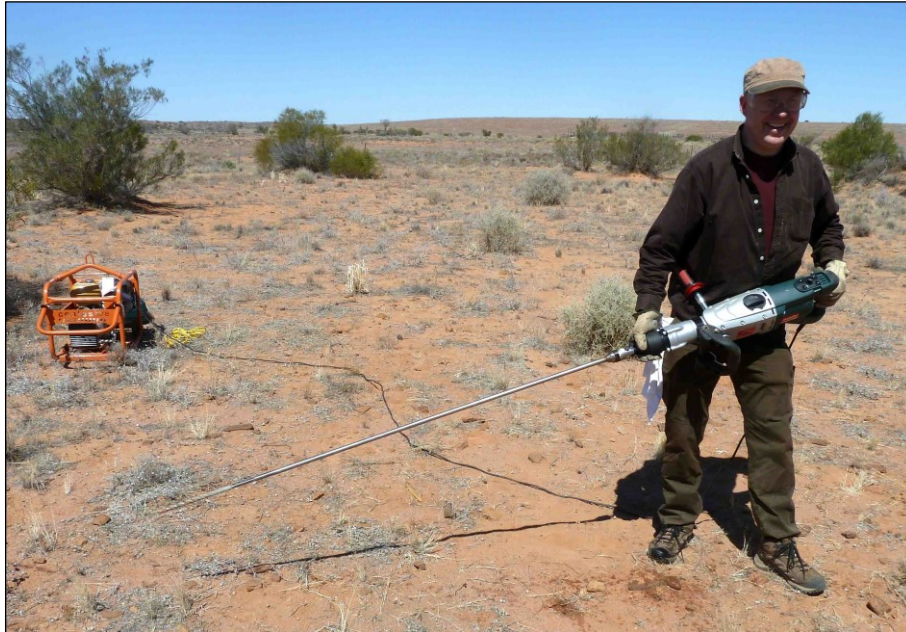
Figure 8: Lawrence Molloy prepares to deploy a Heat Needle at Carrapateena, South Australia.
