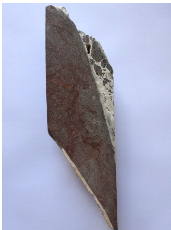
Figure 4: Core sample in sandstones from Buntsandstein at 1204 m deep in the well EPS-1 showing a fracture zone with several individual fractures filled with barite and galena. The diameter of the core sample is 7.6 cm.
