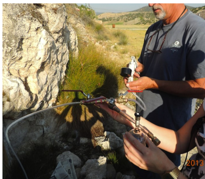
Photo 3: Collection of MMR Gas Sample in Giggenbach Bottle
