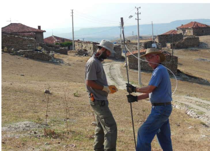
Photo 2: Placement of hollow rods and gas collection tubing
