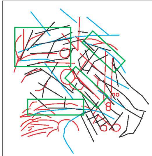
Figure 5: Overlay of structure geology interpretation derived from 2D MT (black line), SVD (blue line), and detailed surface mapping (red line)
