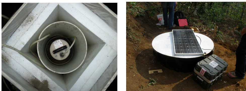
Figure 2: (left) Detail of the set-up of a broad band Güralp seismometer. (right) Station set-up example. The solar panel is fixed on the top of the container where the seismometer is deployed. The box outside contains the EDL data logger (Geophysical Instrument Pool of Potsdam equipment).
