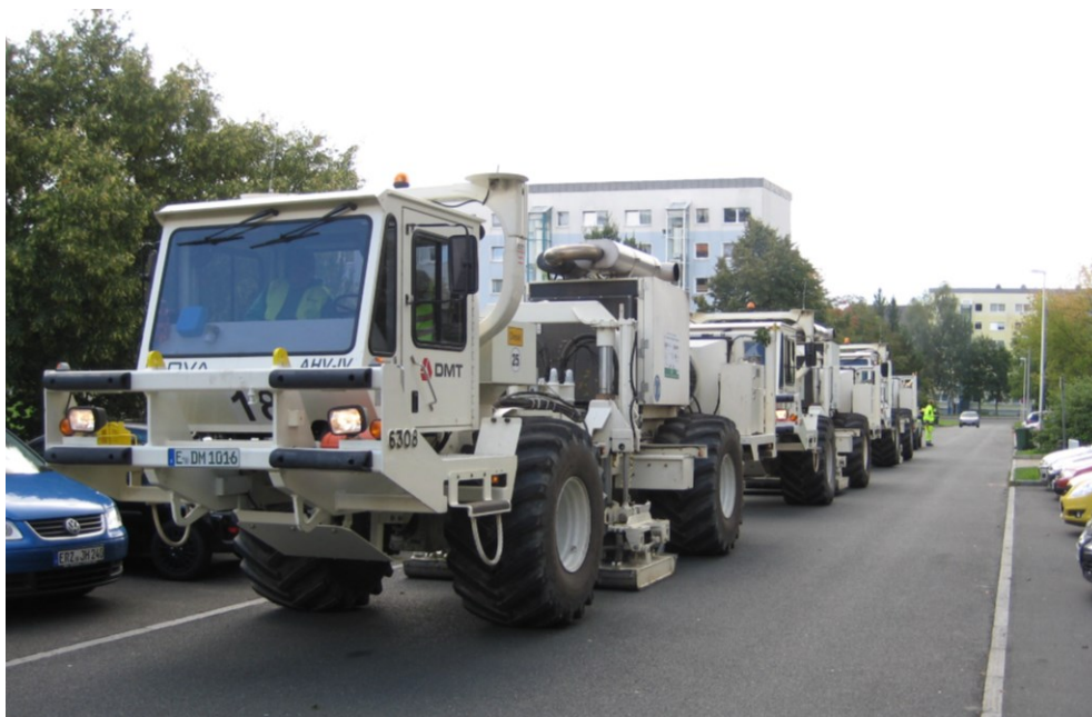
Figure 3: Three 27-ton vibrators as seismic source on municipal roads of Schneeberg (Saxony).
