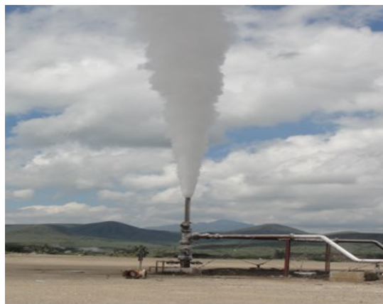
Figure 1: Photo showing OW-38B discharging into the atmosphere. The well has a discharge capacity of 18MW
