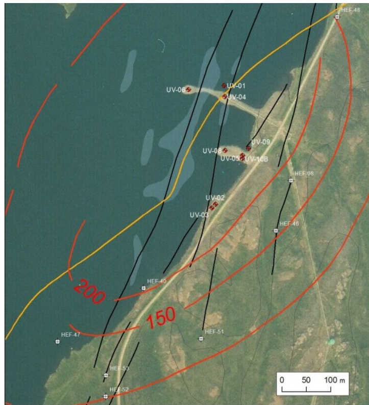
Figure 11. Urridavatn and holes in the ice (light gray shades), temperature gradient (red lines), low resistivity direction (yellow line), intrusions (black lines), UV-boreholes and other boreholes.
