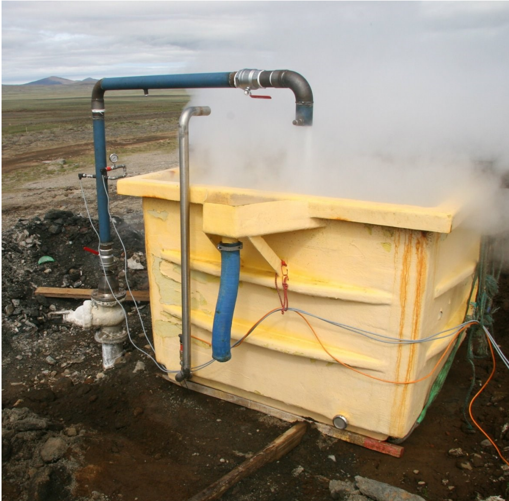
Figure 4: Wellhead setup during the flow test. A 6" tube was directed into the tank, which has a water level indicator.
